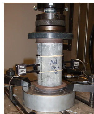
A lightweight concrete test cylinder under compression testing Source: Xb-70 at en.wikipedia [Public domain], from Wikimedia Commons
